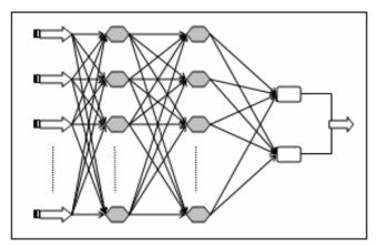
Figure 3. The two-layer perceptron basic architecture.
